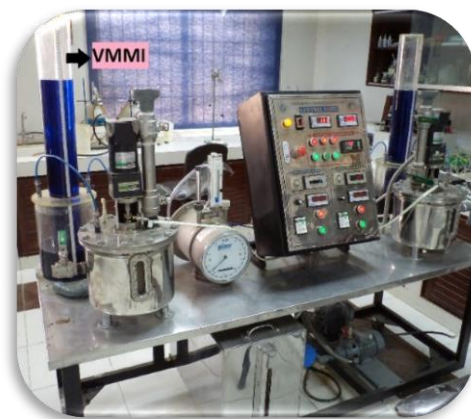
Fig. 2: The developed CSTR assembly for anaerobic co-digestion process optimization
