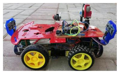
whereas the movement of Robot can be control by using Android cell phone by which we can easily localized the point of leakage. If it detects any traces of gas leakage the buzzer will start alarming and can be hear to the operator, monitoring the robot. So this innovation of tracing gas leakage and monitoring processes improved in the reliability, efficiency and cost effectiveness of inspections.
