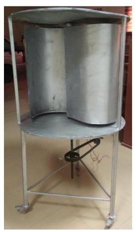
elliptical and semicircular blades to decrease air vacuum and drag to increase the thrust. For the higher efficiency concern we have fabricated combined blade Savonius type vertical axis wind turbine to produce increased power and torque output. The power and torque obtained from the fabricated model at the average wind speed of 8 m/sec are 0.235W and  $4.32 \times 10^{-3}$ .
